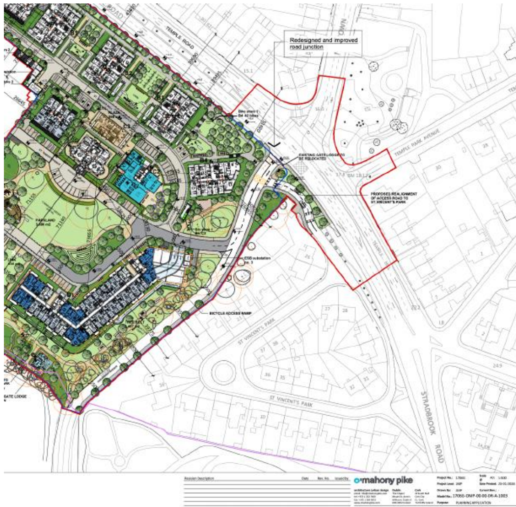
Figure 2 – Extract from the applicant's proposed ground-level site layout showing the D1/B4 side of the development and the adjoining St Vincent's Park residential area. Source: EIAR Appendix 1.1 – Site Layout Plan – Proposed Ground Level, drawing 1706G-OMP-00-00-DR-A-1003. Reproduced as an extract for ease of reference.
